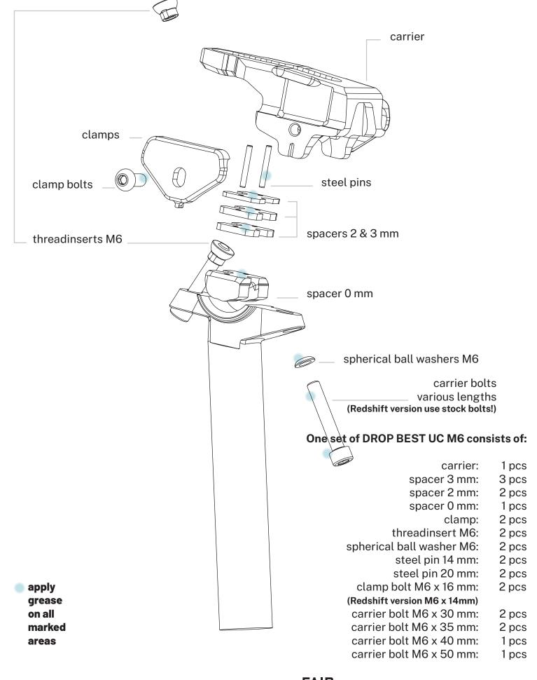
(FOR ALL NON DROPPER, BUT PROPRIETARY POSTS USING M5/M6/M7/M8 HARDWARE)
