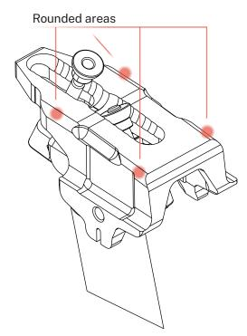
sired. At your selected saddle angle, make sure the carrier bolts engage all threads of the threadinserts and stick out between 1 and 5 mm, using the different length supplied bolts. If the bolts stick out too far, either cut them to the correct length or jump to step \*2. Install the saddle\*, and check whether the saddle at full load (e.g. jumping up from the saddle and dropping your full weight onto it) collides with the bolts sticking out. If it does, shorten the bolts.
